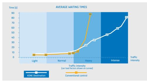
**KONE** Destination combines short waiting times with low car load factors. In traditional control systems waiting times tend to increase exponentially when traffic intensity increases over a critical point, whereas KONE Destination can handle much higher traffic. Builtin artificial intelligence allows KONE Destination to detect periods of lightnormal traffic intensity and adjust the operating mode accordingly in order to optimise waiting times.
