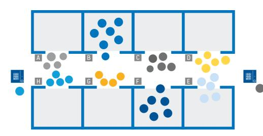
KONE Destination minimises the number of intermediate stops by grouping passengers intelligently. This leads to shorter journey times and better handling capacity compared to conventional full collective lift systems.
