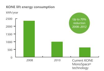
The basis for the calculation is a lift speed of 1 m/s, a load of 630 kg, 150,000 starts/year, a travel height of 9 m and 4 floors
