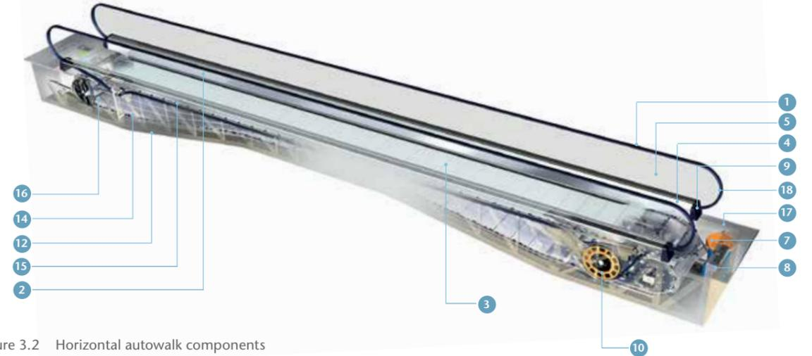
Figure 3.2 Horizontal autowalk components
