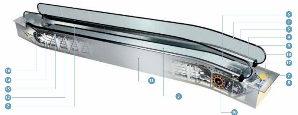
Figure 3.3 Inclined autowalk components
