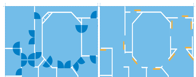
Gliding vs swing doors can save up to 15% of space based on opening area that swing door requires
